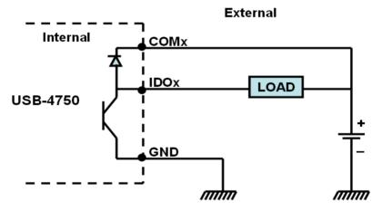
Figure 3.3: Isolated Digital Output Connections
